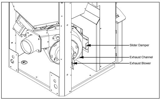
Figure 4: Slider/Damper Plate in Unit.
